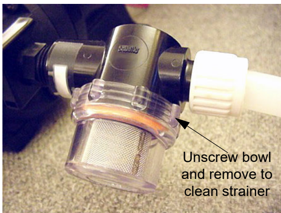
Water Pump Strainer -Typical View
