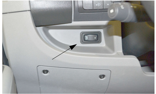
Battery Boost Switch
