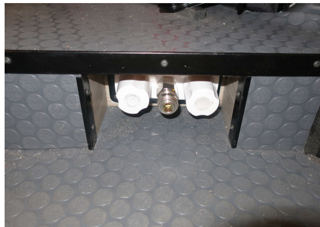
Exterior Shower/Wash Station (located inside passenger main door) - Typical View
