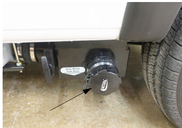
Sewage Drain Outlet (Located beneath motorhome on the left side) - Typical View
