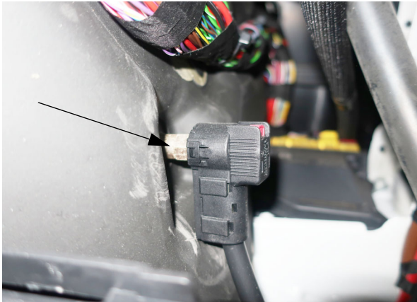
Chassis Battery Connector (Located to the right of the accelerator pedal behind access panel)
