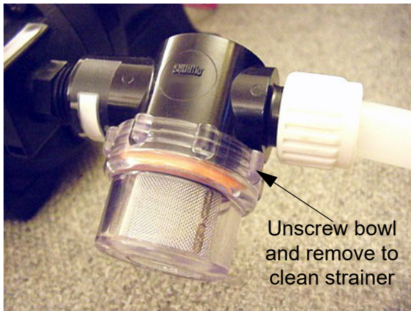
Water Pump Strainer -Typical View
