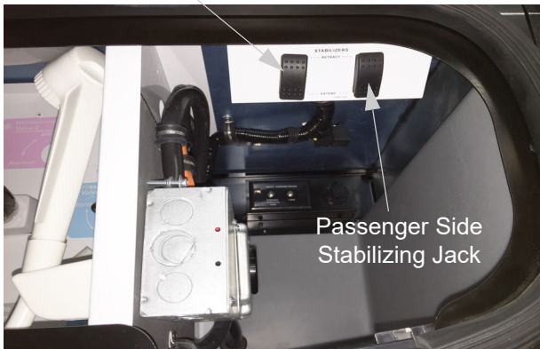
Stabilizing Jack Switches (Located in driver side rear compartment) -Typical View
