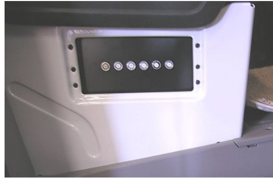
Automotive Chassis 12-Volt Circuit Breakers (Located on outboard side of passenger seat) * Shown with cover removed -Typical View
